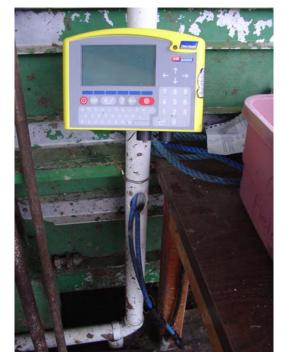
At the South Farm on the Mississippi State University campus, David Pinkerton built a device out of 2-inch PVC pipe to protect the cords running from the load bars of the digital cattle scale to a mount for the digital indicator. The PVC pipe not only protects the cords from damage, but it also keeps them out of the way during cattle working.
