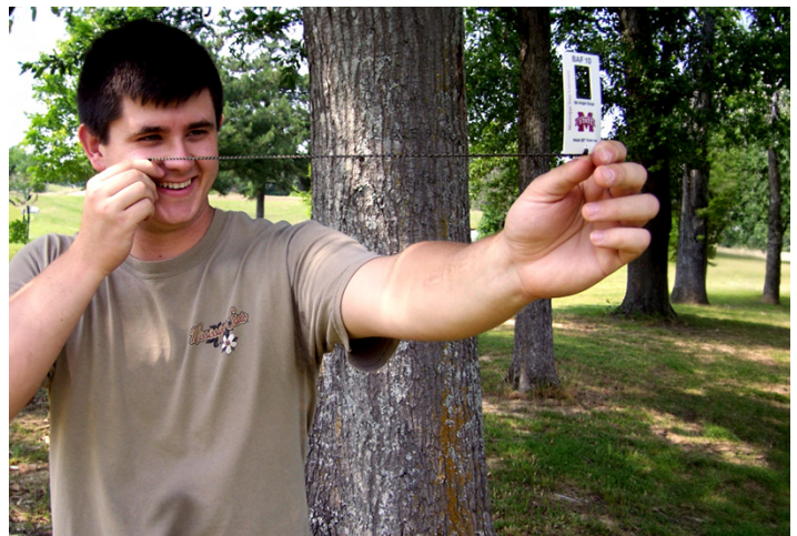
Figure 1. Using the MSU Basal Area Angle Gauge at 25 inches from the eye. Photo by Stephen Dicke.
