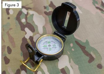
A commercial compass may have other components, too. Not only will one end of the needle be identified as north (or N) and the other south (or S), but typically east and west are identified, as well. A *lensatic compass* allows the user to get a fixed position on a distant object (**Figure 4**) and then determine the *degrees* in which that object is
