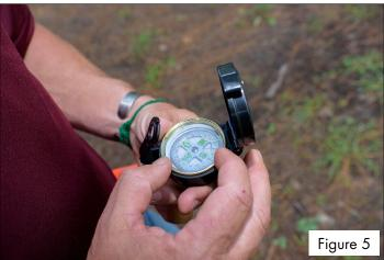
located by using the dial on the face of the compass (**Figure** 5). This is known as *taking an azimuth*. Once you have reached one landmark, then you can take another azimuth to the next landmark, repeating the process until you reach your objective.
