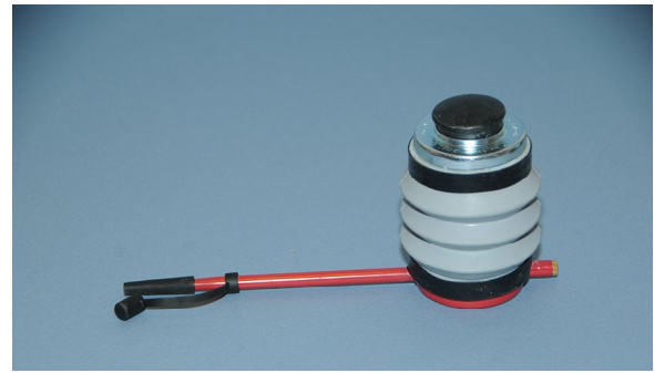
Bulb dusters are useful tools for injecting insecticidal dusts in to cracks, crevices, and voids where spiders seek refuge. Source: Blake Layton, Mississippi State University Extension Service.
